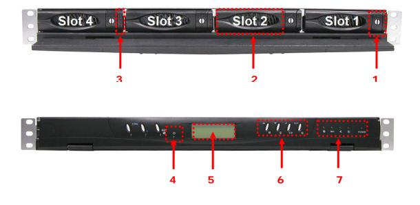
**1 Carrier Open Button** – Use this to open the disk tray. Press the button to open. This button also shows the Lock Indicator.
